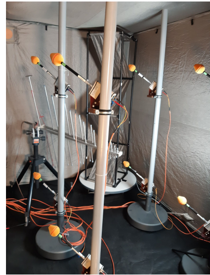
(b) Interior view of the tent-like reverberation chamber with the 8 field probes (orange) and the rotating z-fold mode-stirrer in the background
